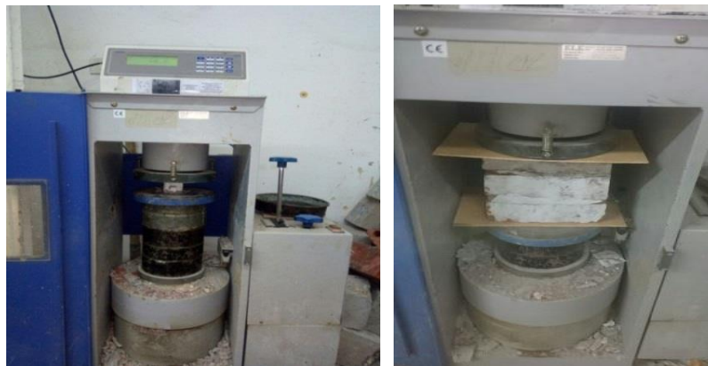
Figure 2 Compressive strength test for mortar cube and for brick prism
