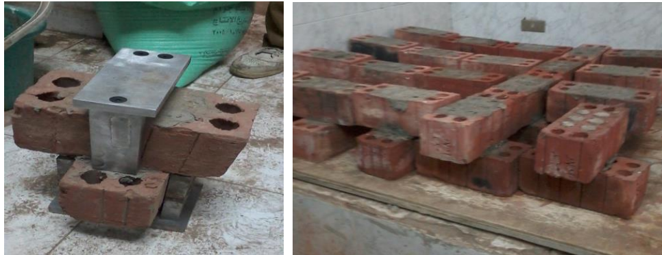
Figure 3 Cross brick specimen for bond strength test and some of the specimens subjected to wetting and drying by water or salt solution
